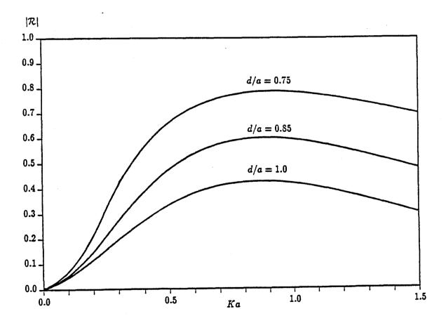
Figure 1: Reflection coefficients for a plate at an angle of  $\pi/4$  to the vertical, plotted against Ka for various values of d/a.
