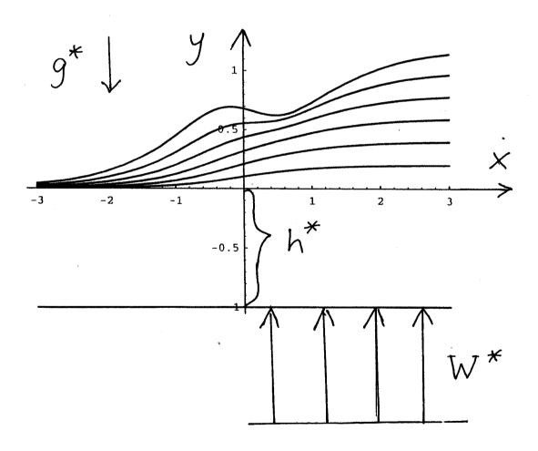
Figure 1: Snapshots of free surface shape  $y=\eta(x,t)$ , to third order in the small-time expansion. Pure upwelling:  $(V_{\downarrow}, V_{\downarrow})=(1,0)$ . F=0.5. Increments of 0.2 are chosen in the dimensionless time t (= t\* W\*/h\*).
