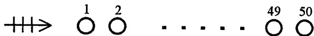
Fig.1 An array of 50 vertical truncated cylinders fixed in waves. (diameter:0.165m,draft:0.215m,distance between cylinders:0.330m,water depth:2.20m)
