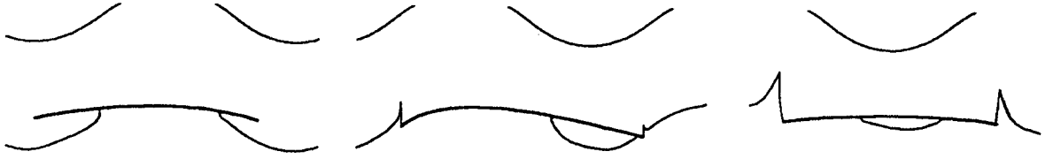
Figure 1: Impact of an elastic beam on a curved liquid free surface. Initially, liquid is at rest, and the elastic plate just touches the free surface. The flow patterns after the impact are shown for different impact conditions (with and without a cavity formation).
