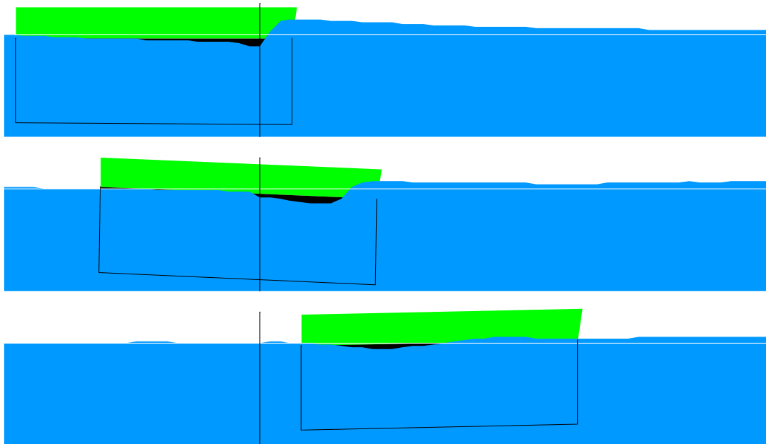
Fig. 3 Calculated ship wave profiles in the lock at three arbitrary instants.
