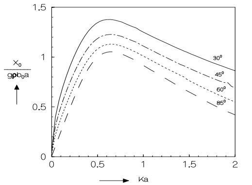
Fig. 3: Amplitude of the force per unit width vs wave number
