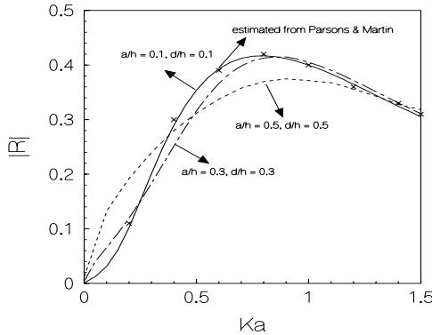
Fig. 1: Reflection coefficient vs wave number,  $\theta = 45^\circ$
