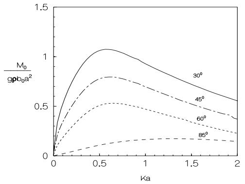
Fig. 4: Amplitude of moment per unit width vs wave number
