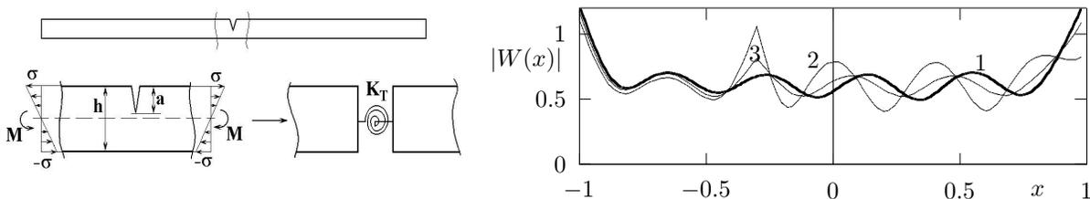
The equivalent torsional spring stiffness  $K_T$  for a single-sided crack is assumed known as a function of the beam parameters and the crack length  $a$ . The 'outer' solution for the floating free-free beam which is divided by the torsional spring into two parts, provides the bending stresses outside the crack region. Therefore the 'outer' solution is described by the problem considered in Section 5, where  $\alpha_1 = \alpha_2$ ,  $\beta_1 = \beta_2$ ,  $k_l = 0$ ,  $k_T \geq 0$ .
