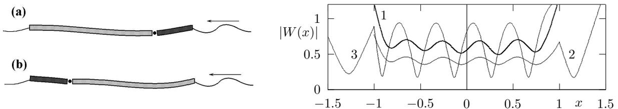
Calculations were performed for the conditions of experiments [8] for main plate. Period of the incident wave is equal to 1.429s (line 1 is for a single plate, line 2 is for case *a*, line 3 is for case *b*, length of the auxiliary plate is equal to 0.25 of the main plate length,  $(EJ)_{aux} = 100(EJ)_{main}$ ). It was revealed that:
