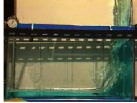
Fig.8 collapse of a dam: t = 0.6
