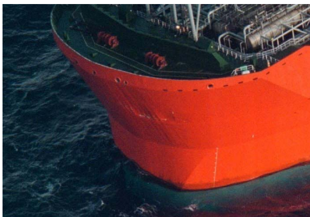
Fig 1. Bow damage on the Schiehallion FPSO
