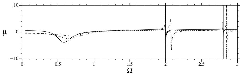
Figure 7: Non-dimensional heave added mass  $\mu$  vs. non-dimensional frequency  $\Omega = \omega/\sqrt{g/h}$  for the structures shown in figure 4: trapping structure (—), pair of half-immersed circles (---), pair of half-immersed ellipses (-·-·-)
