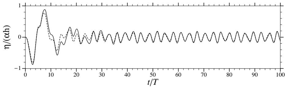
Figure 5: Free-surface elevation  $\eta(0, t)$  generated by the forced motion of the trapping structure (—) and the half-immersed circles (---).
