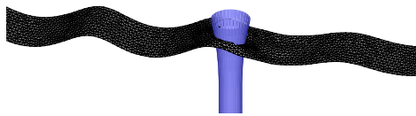
Fig. 8 Wave profile around the flared cylinder
