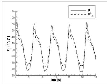
Fig. 10 Comparison between 'strain-gauge' and 'dynamometer' force on the second segment.
