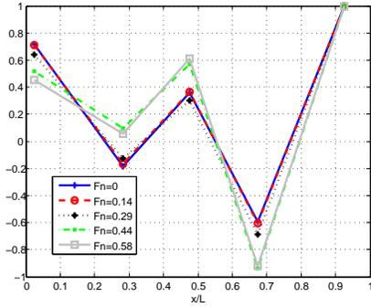
Fig. 5 Modeshape #3 sensitivity to forward speed
