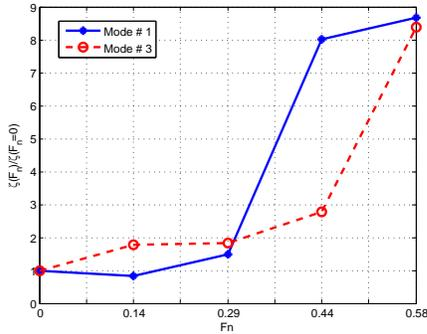
Fig. 9 Damping ratio sensitivities to forward speed
