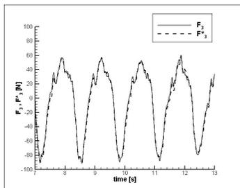
Fig. 11 Comparison between 'strain-gauge' and 'dynamometer' force on the third segment.
