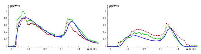
Figure 7: Pressure evolution at the wall locations 0.24f (left) and 0.64f (right) above the deck, with f = 0.05 m the ship freeboard. The water-on-deck has been caused by prescribed regular incident waves  $\lambda = 40f$  long and with a crest-to-trough height  $H = 0.08\lambda$ . Lines with symbols: experiments by Greco (2001), two runs are shown for each pressure sensor. Solid lines: DDDC results. Here t = 0 s the time instant of the initial water-wall impact.
