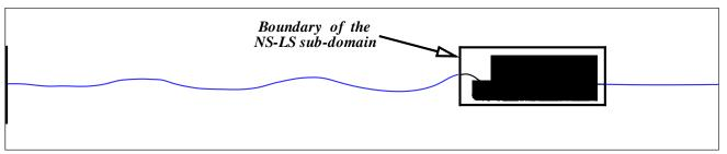
Figure 1: Domain-decomposition strategy applied to the water-on-deck problem. The incoming waves are generated by a flap wavemaker on the left and interact with a ship-like structure. This case refers to the model tests discussed in Greco (2001). The solid box delimits the fluid region described by the NS-LS method. The surrounding sub-domain is solved by the BEM. The horizontal size of the NS-LS region is about 0.08 times the domain extension.
