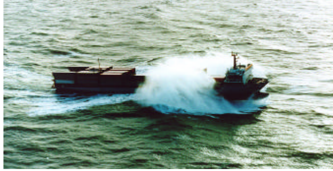
Figure 1. Slamming on a containership in waves (courtesy of American Bureau of Shipping)
