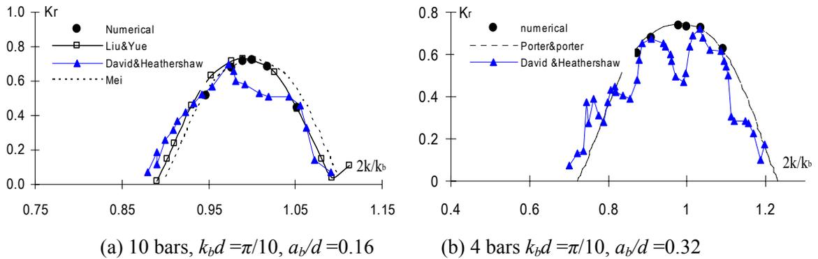
Figure 1 Reflection coefficient as a function of  $2k/k_b$ .
