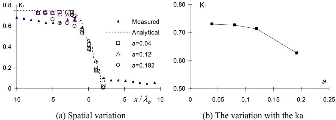
Figure 2 Reflection coefficients with 4 bars in a range of  $-2 < x/\lambda_b < 2$  ( $k_b d = \pi/10$ ,  $a_b/d = 0.32$ )
