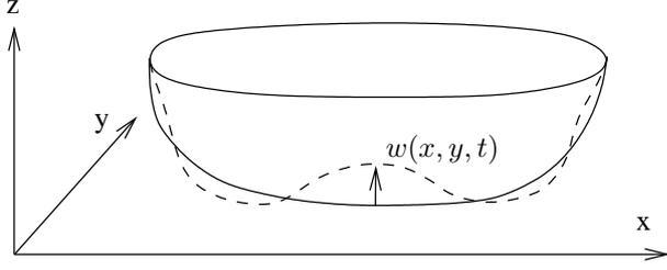
Figure 1: Water impact for a flexible structure
