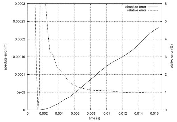
Figure 5: Absolute error (thick line) and relative error (dashed line) between semi-analytical results in [4] and the variational inequality results, for the point  $x=50 \text{ cm}$
