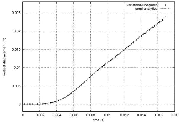
Figure 4: Vertical deflection with respect to time for the point situated at 50 cm of the centre
