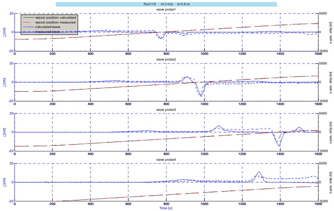
Figure 1, measured and predicted wave in canal configuration
