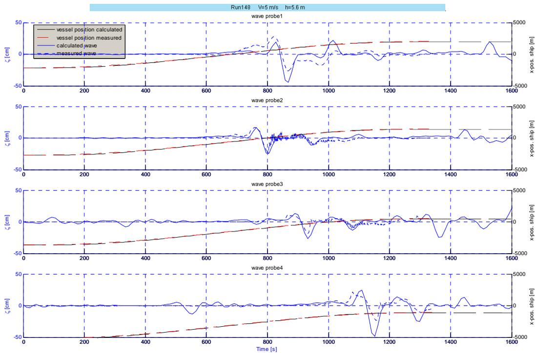
Figure 2, measured and predicted wave in harbour configuration
