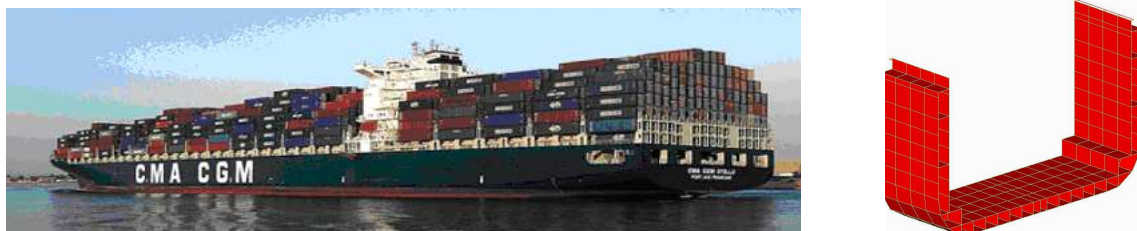
Figure 1: Ultra large container ship and its typical midship section.
