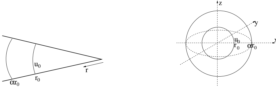
Figure 3: Definition sketches for 2D and 3D axisymmetric air pockets.
